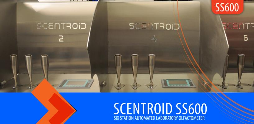
Scentroid SS600 is the world's most advanced stationary, dynamic, and fully automated olfactometer. It is capable of odour measurement and analysis to all international olfactometery standards: EN13725:2003, ASTM E679-04, NVN2820, VDI 3881, GB/T14675-93
