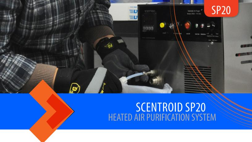
he Scentroid SP20 Heated Air Purification System is a revolutionary device designed to provide an effective and reliable cleaning solution for olfactometers, sample bags, PTFE lines, and other equipment which may be contaminated with odours.
